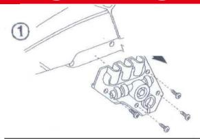
1) Remove the cover (motor dummy) on both sides so that the drive chain and the discs are visible and accessible. On closer inspection you discover the excentric position of the axles in the disc.
