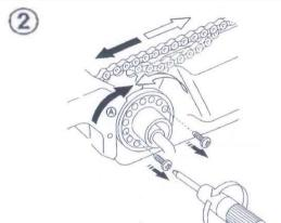
2) Dismantle both screws of the disc and turn it towards the seat till the drive chain has enough tension again.
